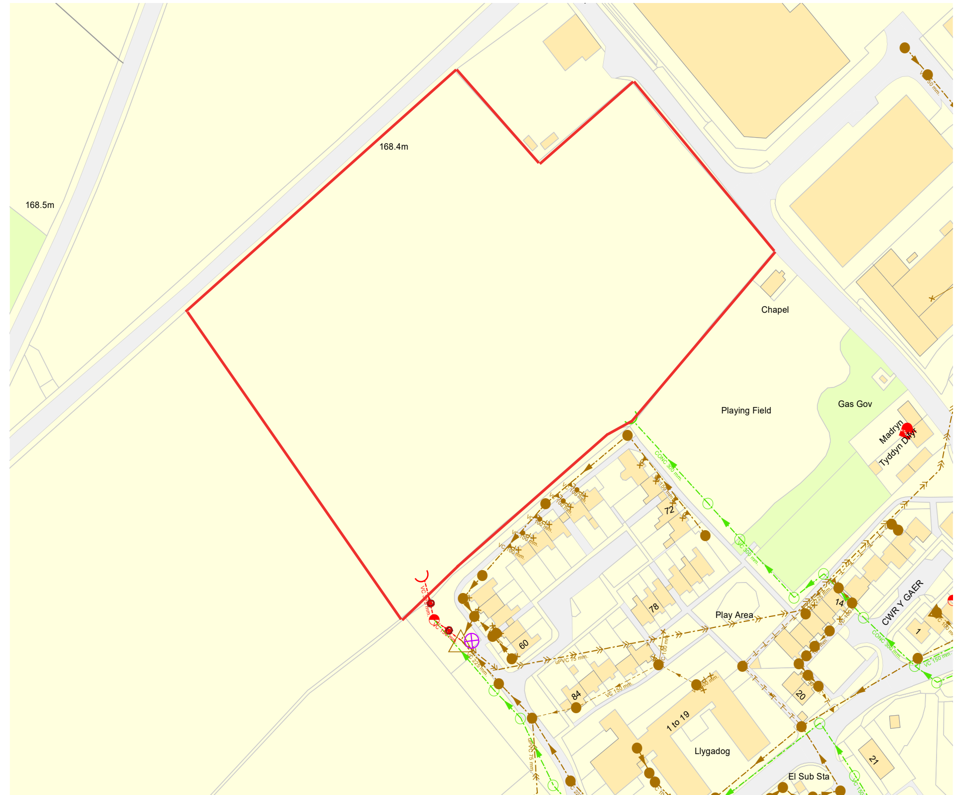
Figure 4 Dwr Cymru Welsh Water Sewer Records Extract
