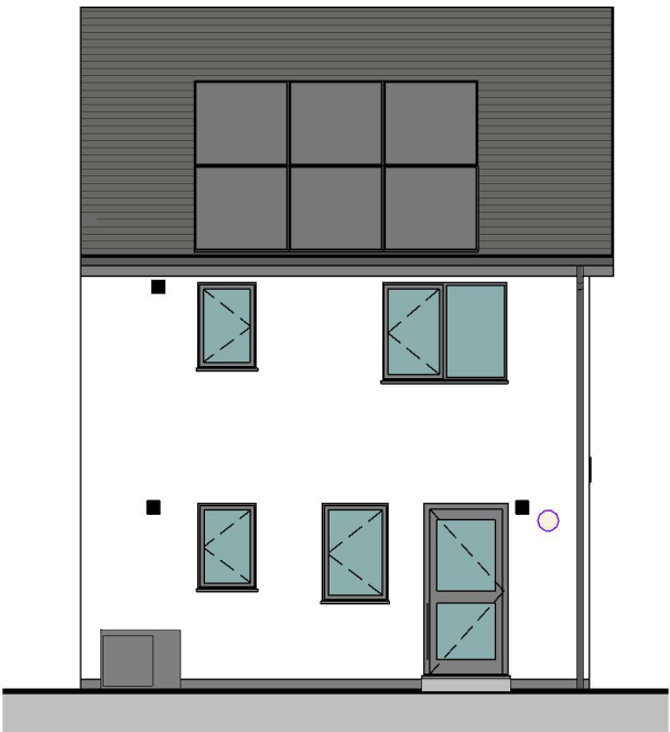
PV's TO REAR OF PLOT:#21
