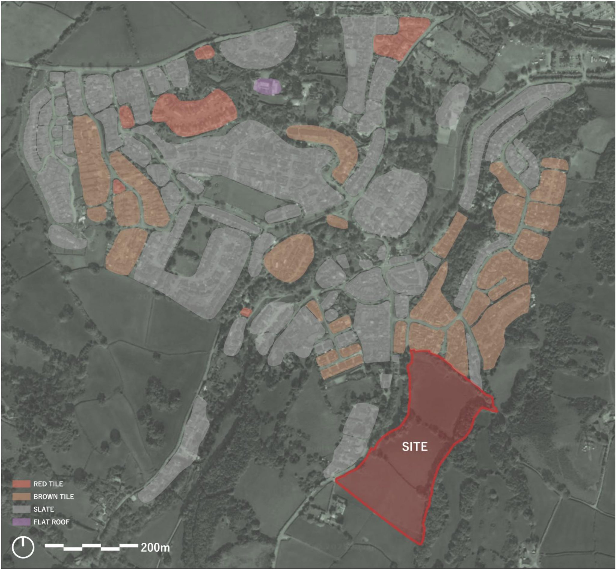
Image 1 - Roof materials analysis
