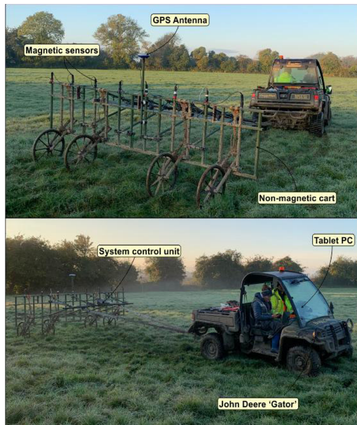
Plate 5: John Deer Gator and Sensys Magneto MXV3 (Library photo).
